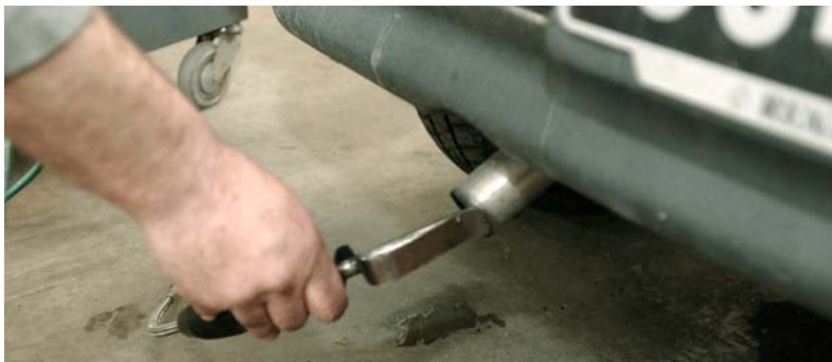
A car's particle emissions being measured during a periodic vehicle test
