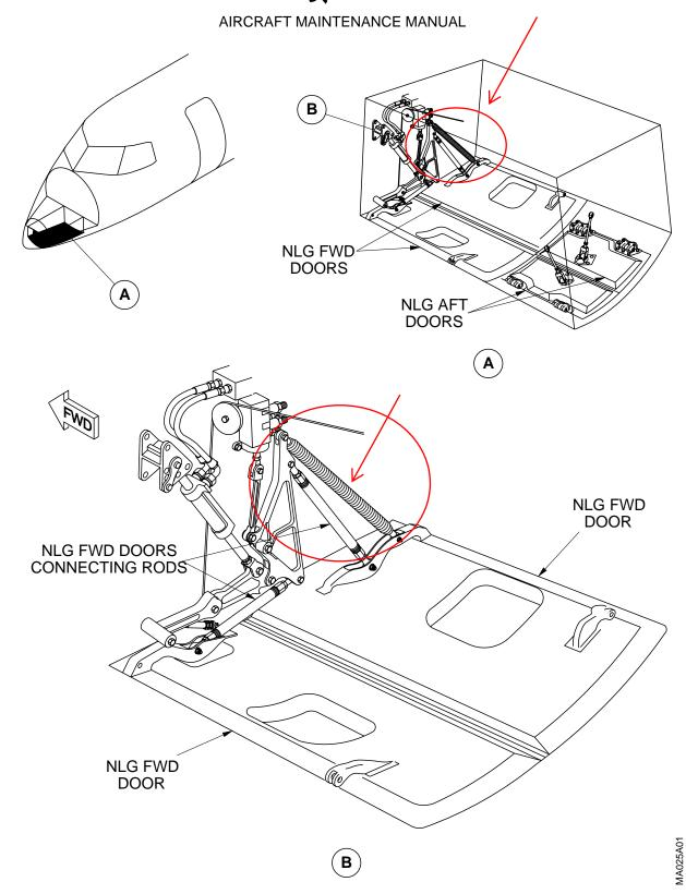
Nose Landing Gear Doors – Component Location
