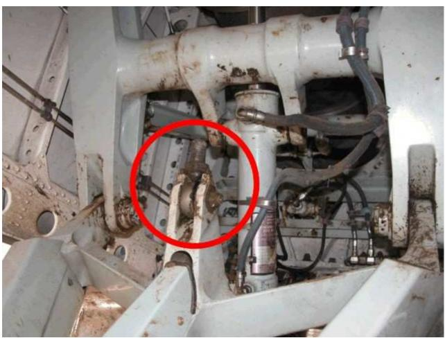
Figure 1: View of separated rod end.
