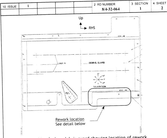
View looking fwd on debris guard showing location of rework
