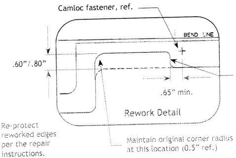
Re-profile lower edge of debris guard to the maximum dimensions shown.
