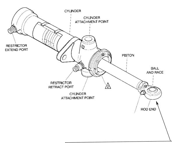
Remove the rod end of the retraction actuator assembly in accordance with SCR 086-07 rev. D
