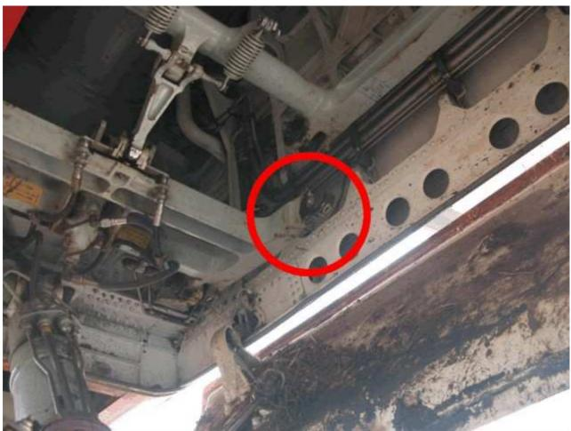
Figure 2: View of broken stabilizer brace assembly.
