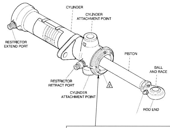
Remove the rod end of the retraction actuator assembly in accordance with SCR 091-07 rev. NC
