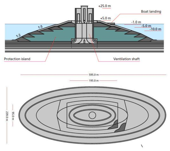
Figure 2.6 Ventilation island of the immersed tunnel solution
