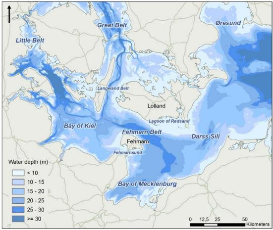
Figure 3.4 Bathymetry of Fehmarnbelt and the surrounding region
