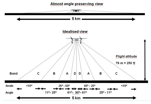
Figure 7.13 Methodology for aerial surveys: division of the transect sections.
