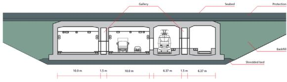
Figure 2.5 Cross section of the suggested immersed tunnel solution
