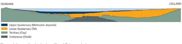
Figure 3.3 Geological profile of Fehmarnbelt
